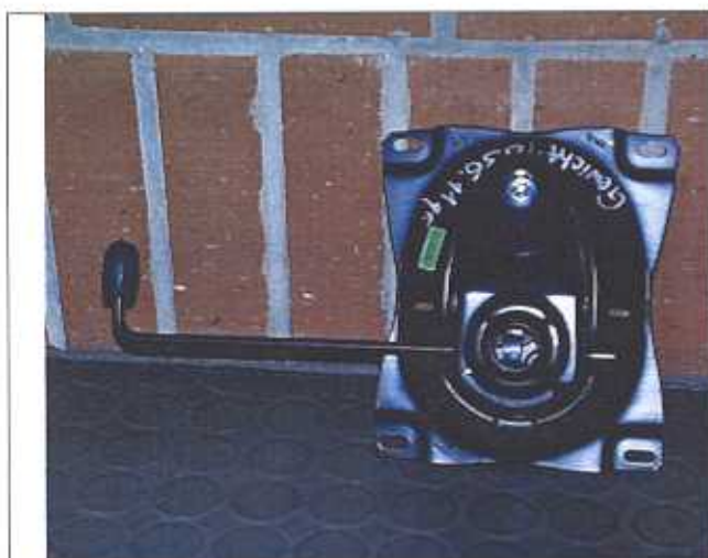
Photo 1 : Seat mechanism model X117CV LGA-reg 450-2 visible side when built in the office work chair
